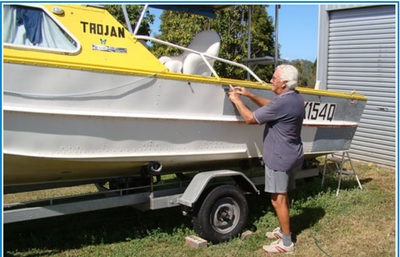
One of Neil's summer jobs ("when the wind is too strong to fish") is to refurbish the hull paint on the Trojan, a task that is surprisingly difficult for an amateur to handle - especially on a rivetted hull like this. Regular paint strippers were ineffective, sanding discs are problematic on and around the rivett heads, so paint stripper combined with an old fashioned paint scraper and lots of elbow grease proved the best - albeit painstaking - solution.
