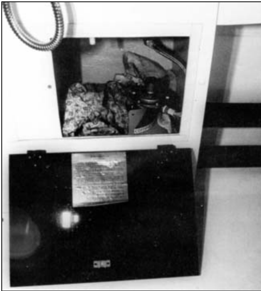
The LP gas bottle is located in this special locker in the cockpit.
